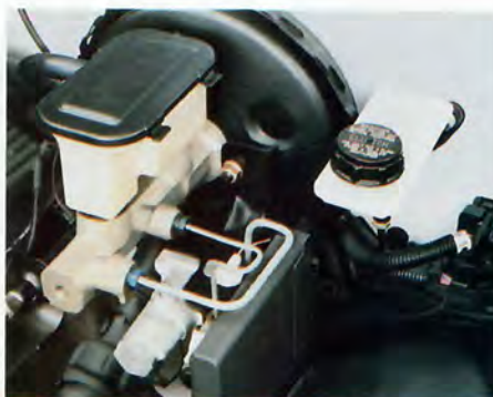
Rear wheel anti-lock brake control unit
