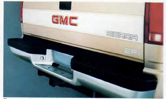
Rear step bumper/platform trailer hitch in trailer package
